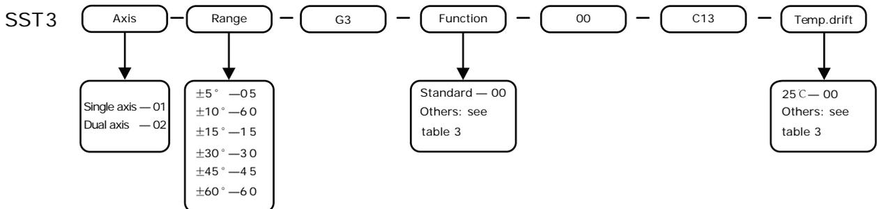
For example, if order a dual axis CAN inclinometer, with range  $\pm 15^\circ$ , room temperature accuracy  $\pm 0.02^\circ$ ,  $-20\text{--}60^\circ\text{C}$  accuracy  $\pm 0.02^\circ$ , output CAN2.0, 25 meters cable with plug, GPS function module, the model should be chosen as: SST302-15-G3-F1-00-C13-D3 (25m)
